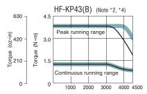
Notes: 1. For the servo motor without reducer. 2. For 1-phase 230VAC. 3. --- : For 1-phase 100VAC -: For 1-phase 200VAC. The line is drawn only where differs from the other two lines
