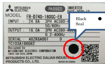
Photo (5) MDI INV Body Rated Label 5.5 kW or More (nameplate label model)
