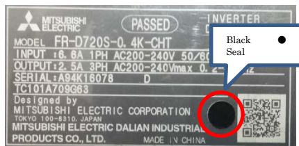
Photo (4) MDI INV Body Rated Label 3.7 kW or Less (laser impression machine)
