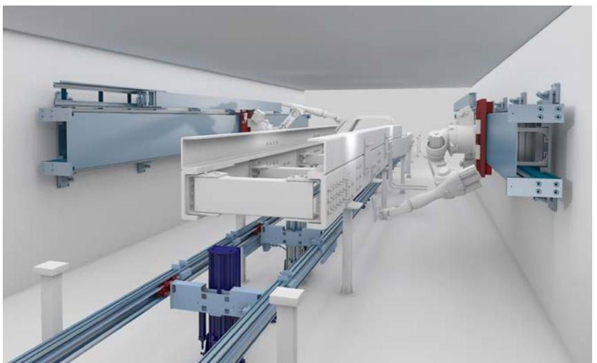
There are several things to consider when designing a 7th axis for a robotic arm. Placement, mounting surfaces, clearance space, speed, and maximum load must be designed for prior to picking the actuator rails.
