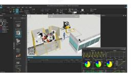
Pre-verification is performed in the digital space of a virtual factory or equipment line. This significantly reduces cost and time during the design phase.
