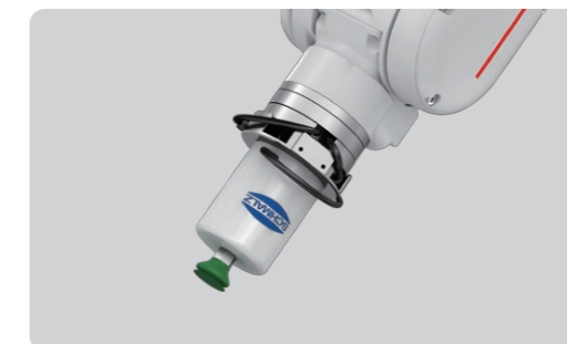
ROB-SET ECBPM ASSISTA(SCHMALZ) Electric-powered Adsorption Gripper
