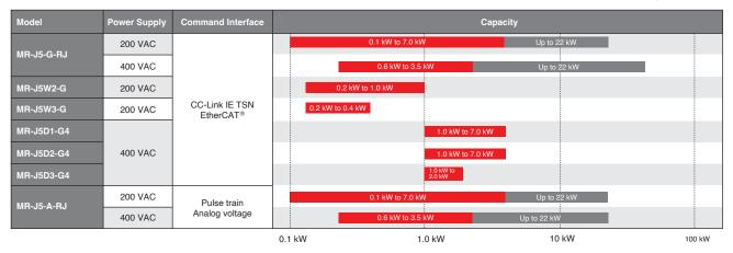
Notes: 200 VAC servo amplifiers are compatible with DC power supply input as standard The indicated servo amplifiers are compatible only with a two-wire type serial encoder. For four-wire type serial encoders and pulse train interface (A/B/Z-phase differential output type) encoders, use MR-J5-G-RJ/MR-J5-A-RJ servo amplifiers. EtherCAT<sup>®</sup> is supported by MR-J5-G-N1/MR-J5W3-G-N1 servo amplifiers.
