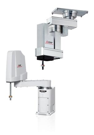
With consumer needs rapidly evolving towards increased diversification and reduced time to market, today's manufacturers face a time of considerable change. It is no longer enough for industrial robots to simply perform a single task. The RH-FRH Series horizontally articulated SCARA robot provides new, intelligent solutions, offering a simple approach to advanced and flexible production.
