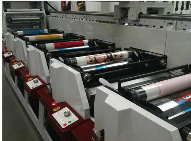
*“The iQ Automation Platform and MR-J4B-RJ Servo System from Mitsubishi Electric improved our tension control by 500%, with more accurate registration and less servo following error than other systems we have tested.”*
