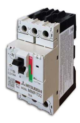
MMP-T32 integrates low voltage circuit breakers and thermal overload relay functions. This device is capable of protecting the motor branch circuits from overload, phase-loss and short-circuit occurrences. The MMP-T32 enables more secure wiring and motor protection than standard open type starters.
