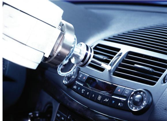
to compare testing quality and conditions from location to location. With Battenberg's haptic system, OEMs and suppliers simply share the program. Battenberg's location-independent, reproducible measurement results also allow standardization of quality features, which overcomes the challenges of global quality evaluations. "We eliminate obstacles and close the loop between suppliers and OEMs," comments Battenberg.
