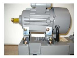
Brackets (2-piece set) for mounting the XC-GMFY to the XL-554-20Y Part #K14M72354101)
