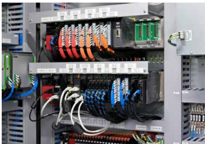
The first steps in electrification and digitalization of the filling machines was the use of PLC control. This expanded to servo systems as they evolved to develop electronic cam functions.
