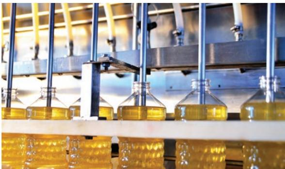
Mitsubishi Electric's iQ-R motion controller intelligently controls cam profiles. Our flexible software system replaces hardware-based methods, which are prone to deviation and error. If the bottle type changes, you can simply exchange the software, even while the system is in motion.
