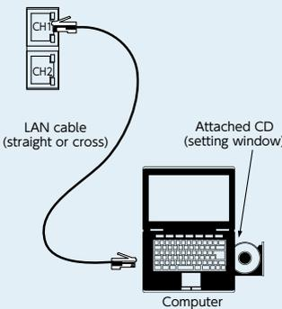
When connecting the PLC (CH2)
