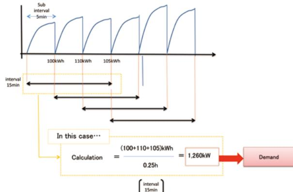
**EcoWebServer III with demand monitoring function comply with the Fixed block demand management method. Interval can be selected from 15min or 30min or 1hour.**
